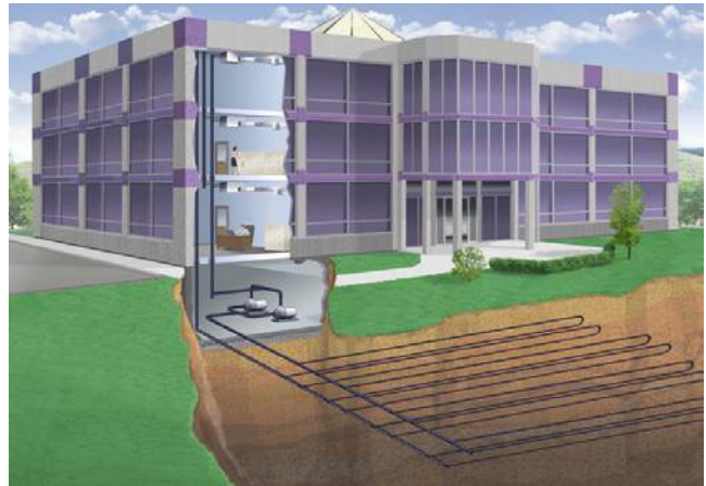
Figure 27: Horizontal Loop Application
