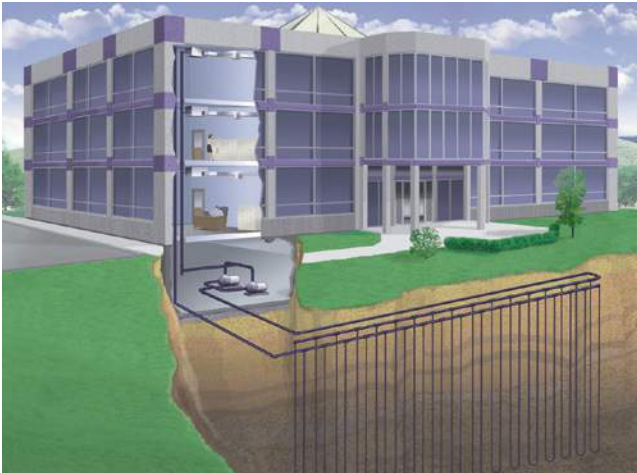
Figure 26: Vertical Loop Application
