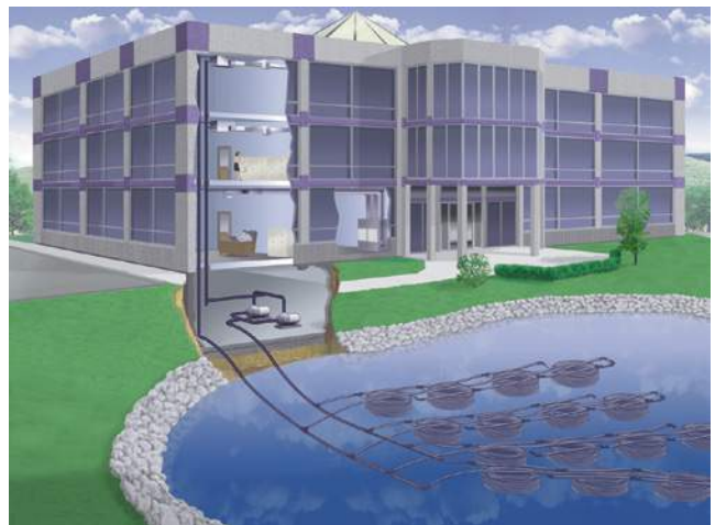
Figure 28: Surface Water Loop Application
