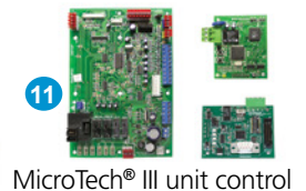
MicroTech® III unit control
