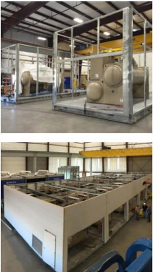
Each modular central plant is custom designed and fabricated in our production facility by our certified team for your specific project. Engineered with the most efficient and highest performing components and materials, your MCP is ready to deliver savings. Before shipping to your site, each MCP is fully assembled and tested in the factory as a complete central plant.
